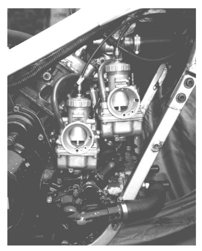
Figure 32: VM34 mounted to the engine
