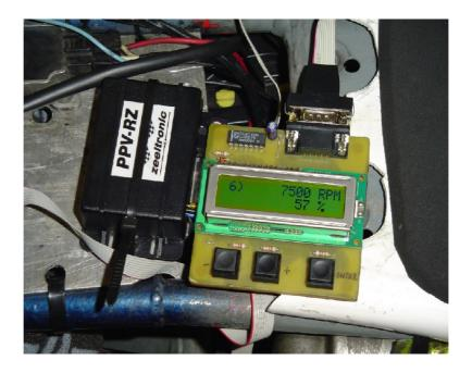
Figure 92: PPV mounted on my Race RZ350 (Handheld is a prototype)
