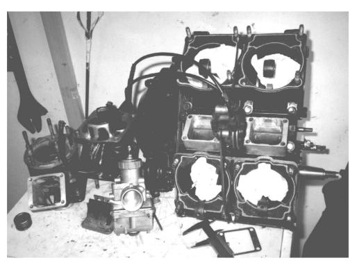
Figure 31: Engine view (sleeve mods, reed cages, reed housing lower cylinder bank)
