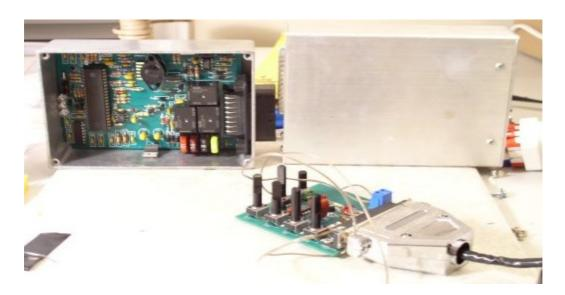
Figure 34: Steve's MiniMegaSquirt ECU (testing with stimulator board)
