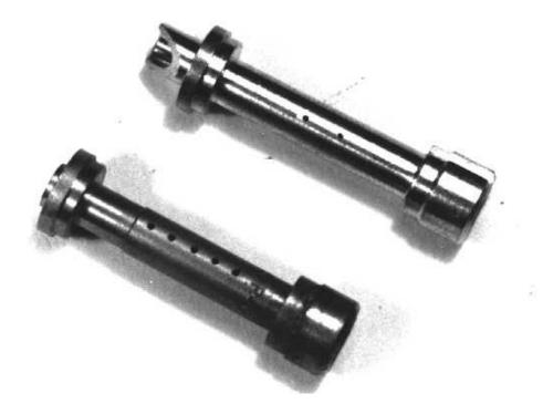
Figure 17: Nozzles, front RD350 O-0, rear: Ledar intake kit
