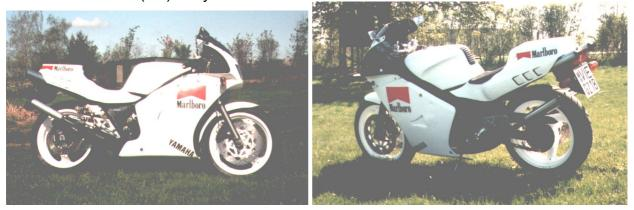
Figure 106: Klöpper RD500 (FZR conversion, RGV Bodywork, Jolly pipes)
