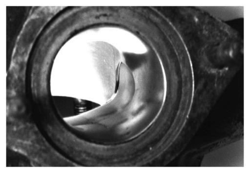
Figure 70: Exhaust port machined and polished (RD350)
