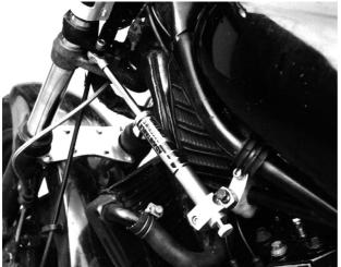
Figure 102: Steering damper (RD350)
